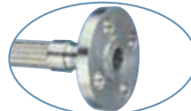
Flange Retainer, Lap-Joint Style Style 12 Lap-joint forged flange per ASTM specifications Schedule 10 Type "C" stub ends & 150# epoxy coated carbon steel lap-joint flanges standard. Consult factory for optional stainless steel flanges and alternative stub end types/schedules
